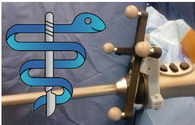
scikit-surgerynditracker is a python interface for Northern Digital (NDI) trackers. It should work with Polaris Viera, Spectra, and Vega optical trackers and Aurora electromagnetic trackers. Tracking data is output as NumPy arrays.
